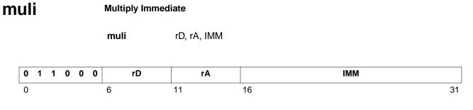
Multiplies the contents of registers rA and the value IMM, sign-extended to 32 bits; and puts the result in register rD. This is a 32-bit by 32-bit multiplication that will produce a 64-bit result. The least significant word of this value is placed in rD. The most significant word is discarded.
